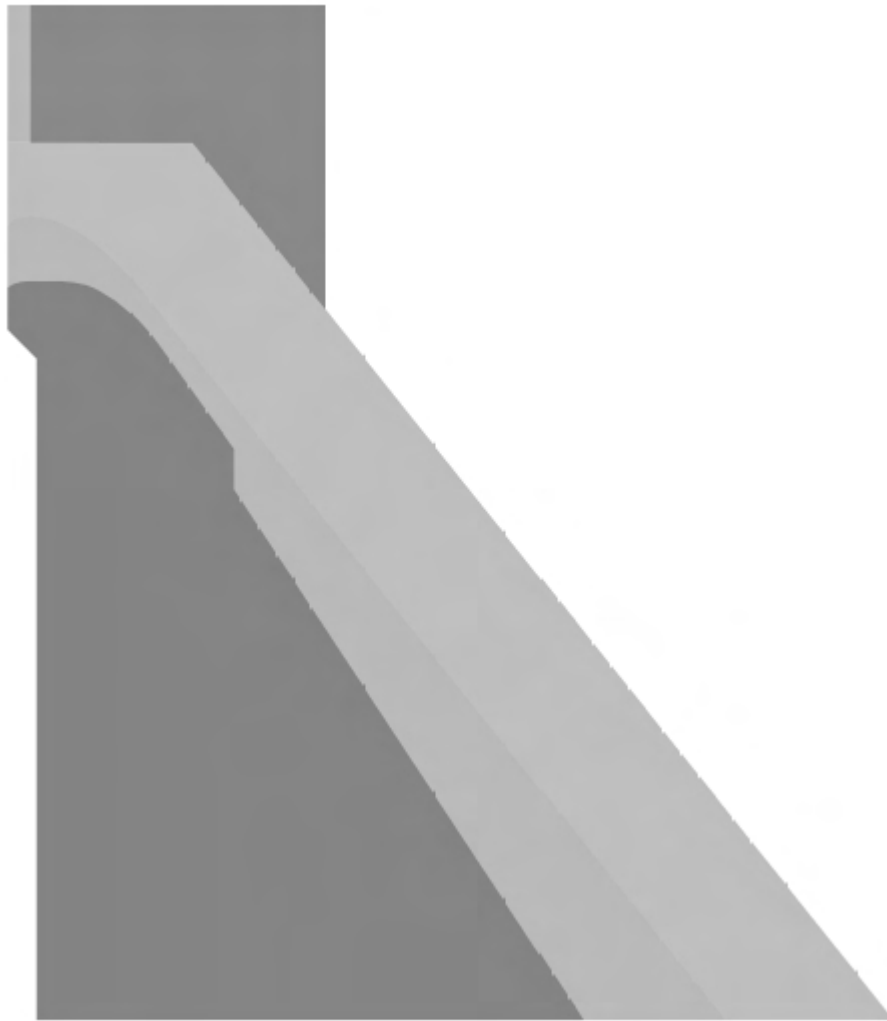
Figure 6-3: Section through labyrinth spillway
