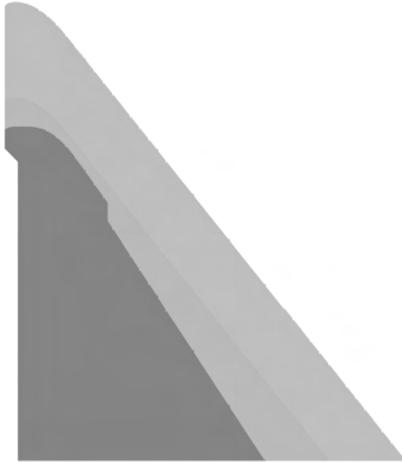
Figure 6-2: Section through ogee spillway for 10 m raising
